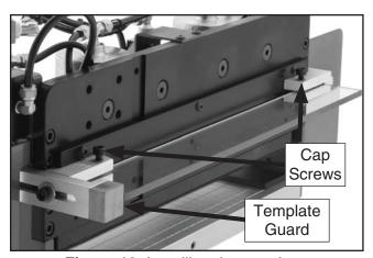
Figure 13. Installing the template.
